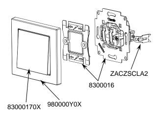
Figure 1. Single one-way rocker switch
